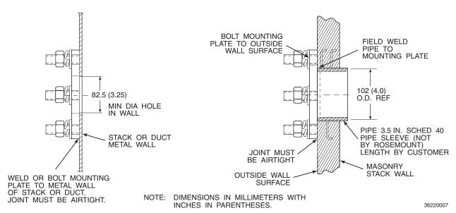
Figure 2-4. Hazardous Area Oxymitter DR Adapter Plate Installation
